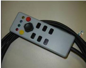
Fig.3 Developed input device for operating a service robot
